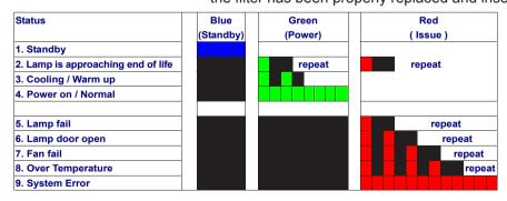
Remark: error codes can easily be read out through projector toolset ( rs 232 or ip ) and via web browser. Remark: The time period of each step in the above LED blinking pattern is 500 milliseconds, e.g., for"Cooling / Warm up"state, the green LED will ON for 500 milliseconds, and then OFF 500 milliseconds, and then repeat the above LED pattern.
